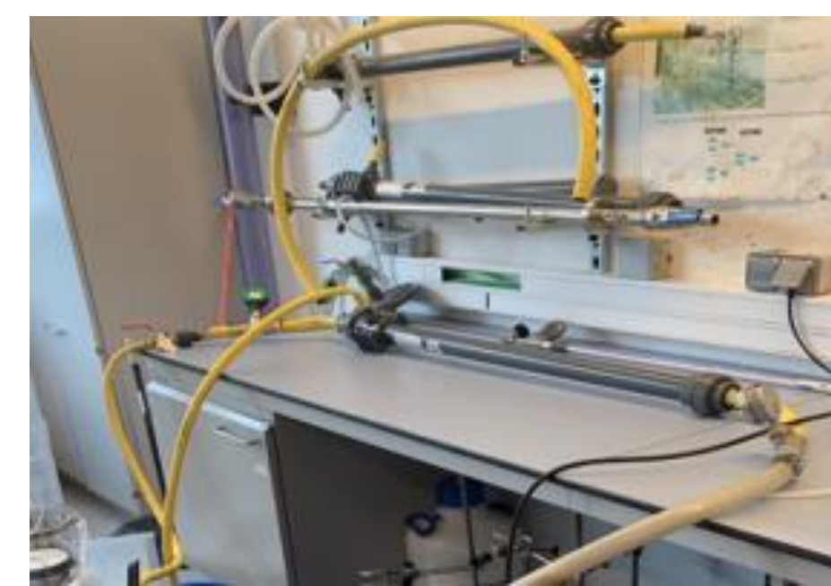
Figure 4. Tubular UF membrane set-up at lab scale
